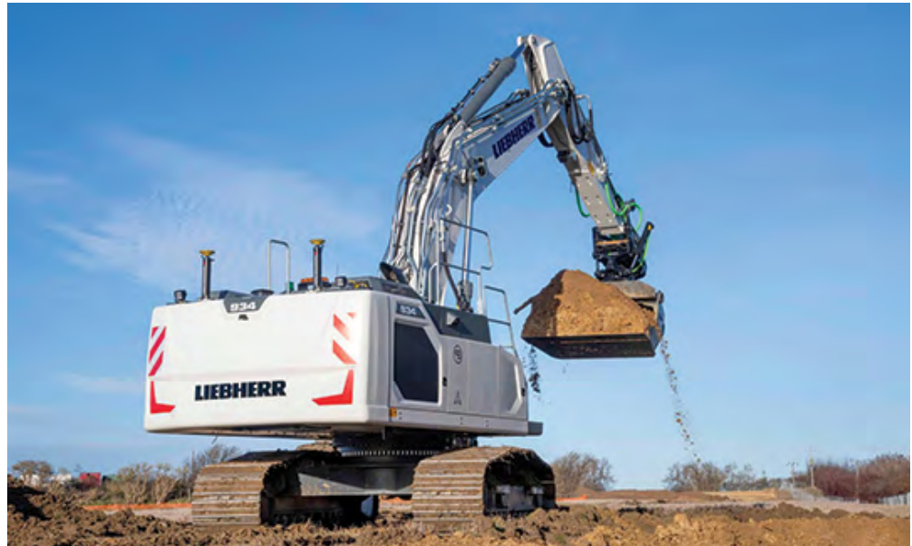
A Liebherr R 934 G8 crawler excavator, the first hydraulic excavator with a factory-fitted Leica Geosystems machine control system, has been delivered to a customer in the UK.
