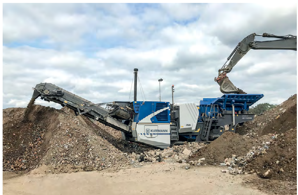
The MOBICAT MC 110(i) EVO2 is designed for the first crushing stage and is used to crush medium-hard to hard natural stone, and in recycling.
